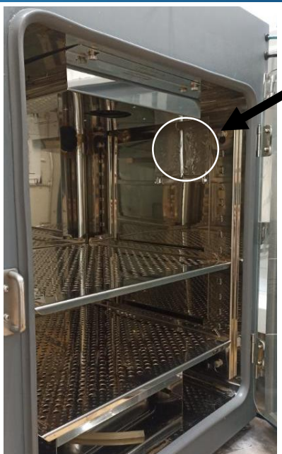
Figure 2. Area with the lowest temperature in the chamber (Top-Right Front) of the Esco CelCulture® CO 2 Incubator with High Heat Sterilization® CO 2 Incubator
